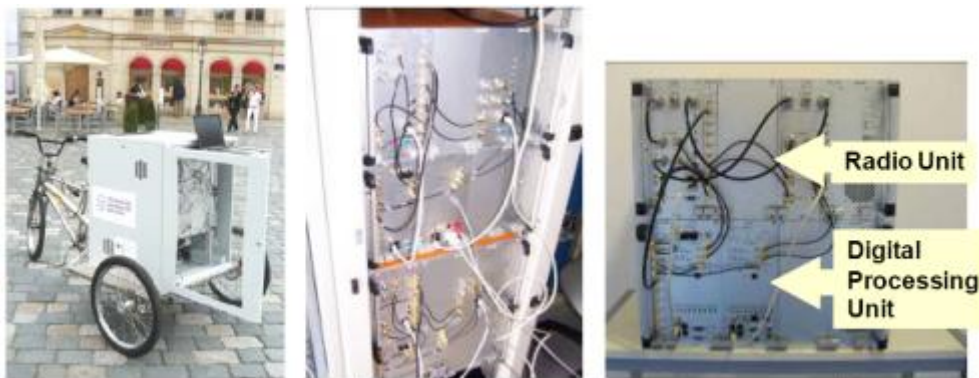
Figure 1 LTE-LTE-A testbed equipment: a) mobile test UE, b) base station equipment, c) UE lab equipment.
